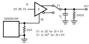
Figure 8. TRI-STATE Test Circuit (t<sub>PZH</sub> , t<sub>PHZ</sub>)
