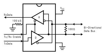
Figure 18. Typical Pin Connection
