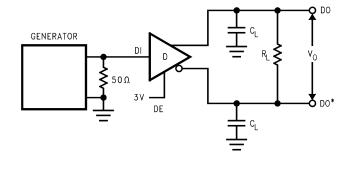
Figure 6. Driver Differential Propagation Delay Test
