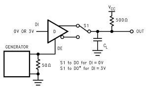
Figure 10. TRI-STATE Test Circuit (t<sub>PZL</sub>, t<sub>PLZ</sub>)
