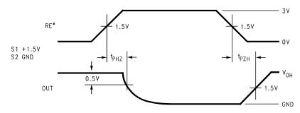
Figure 17. Receiver Enable and Disable Waveforms ( $t_{PHZ}$ ,  $t_{PZH}$ )
