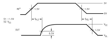
Figure 16. Receiver Enable and Disable Waveforms (t<sub>PLZ</sub>, t<sub>PZL</sub>)
