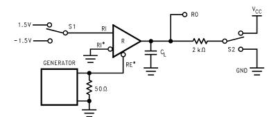
Figure 15. Receiver TRI-STATE Test Circuit
