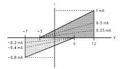
Figure 19. Input Current vs Input Voltage Operating Range
